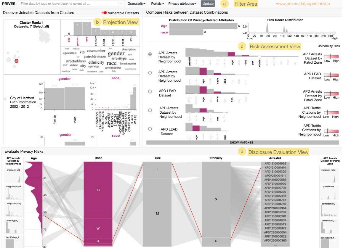
Figure 4.2 Interface Design: The design of PRIVIEE comprises rich interaction among filters and multiple views: (a) Filter area helps select datasets based on metadata like tags, data granularity, and privacy-related attributes; (b) Projection View lets the defenders compare the signatures of different joinable groups of datasets and evaluate vulnerable data distributions; (c) Risk View helps compare the risk for dataset pairs and select the high-risk pairs; (d) Disclosure Evaluation View helps to analyze the matching records for potential disclosures.
